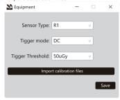
Step 3: Find the file called "Calibration File" in the USB flash disk to import all three calibration files.
